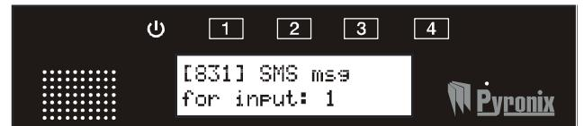
Enter the text message using the relevant keys (see page 6 for help on entering text). A maximum of 160 characters may be used. Press
