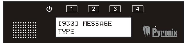
Press or to select which message type for which telephone number needs to be programmed (or enter the programmed function number).
