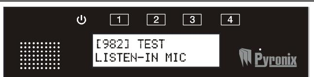
The V2 GSM is now testing the Microphone, press **X** to stop the test.
